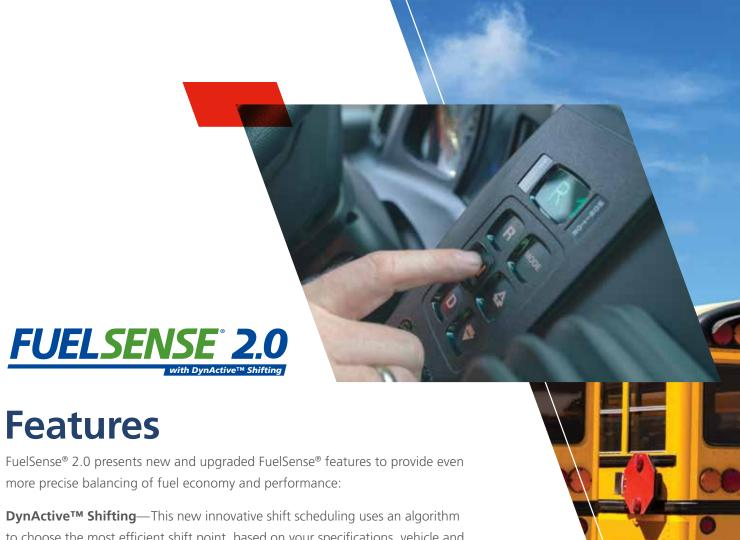
**DynActive™ Shifting**—This new innovative shift scheduling uses an algorithm to choose the most efficient shift point, based on your specifications, vehicle and environmental parameters. Older shifting technologies use shift schedules with fixed shift points.
